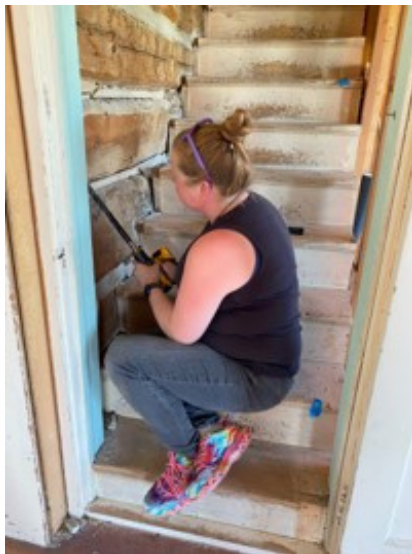
Picture of Dr. Lauren Stachowiak collecting a core from a beam in the interior stairwell of a historic structure. The core has tree rings which are used to reconstruct the calendar year in which the structure was built.
